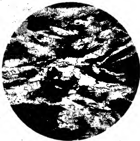
FIG. 90.—MICROSTRUCTURE OF COLD WORKED STEEL AFTER RE-HEATING TO 540° C., SHOWING THE SPLITTING UP OF THE FERRITE GRAINS, \times 400 DIAS.
