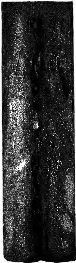
FIG. 21.—SULPHUR PRINT OF A ROLLED BAR SHOWING SEGREGATION OF SULPHUR IN AXIS OF BAR.
