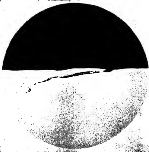
FIG. 102.—SECTION OF STEEL THROUGH A CRACK, PRODUCED DURING HEAT TREATMENT, AND STARTING AT THE BASE OF A FORGING LAP.
