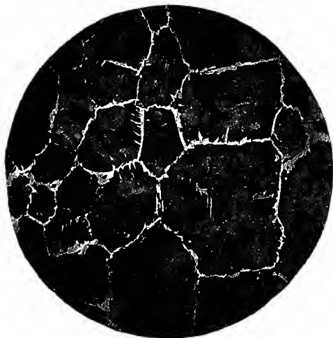
FIG. 94.—MICROSTRUCTURE OF PATENTED STEEL BAR, \times 300 DIAS.
