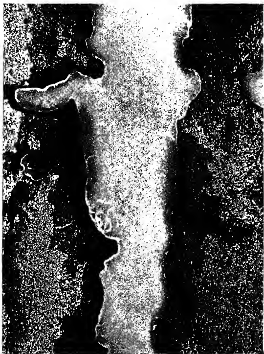
FIG. 20.—SULPHUR PRINT OF SECTION OF AN INGOT THROUGH AXIAL PIPE.
