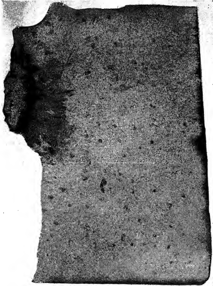
FIG. 22.—SULPHUR PRINT OF FORGING SHOWING FRACTURE THROUGH REGION HIGH IN SULPHUR (DARK AREAS ARE THOSE HIGH IN SULPHUR).
